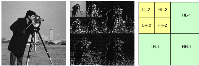
Fig. 10. Wavelet decomposition of an image at scale 2.
